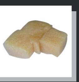
Styrene-Butadiene Rubber (SBR) consists of about 25% styrene, with butadiene making up the rest. It has similar properties like natural rubber. This rubber is a widely used synthetic rubber known for its abrasion resistance, high tensile, impact strength, and resilience. It's flexible in low temperatures has decent heat resistance as well. SBR is water, organic acid, ketone, chemical, alcohol, and aldehyde resistant.
